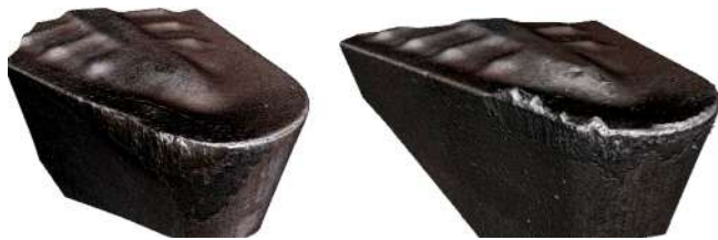
Fig. 15. 3D scanning of the inserts after machining. a. Inconel 718-oil emulsion; b. Haynes 263-oil emulsion.
